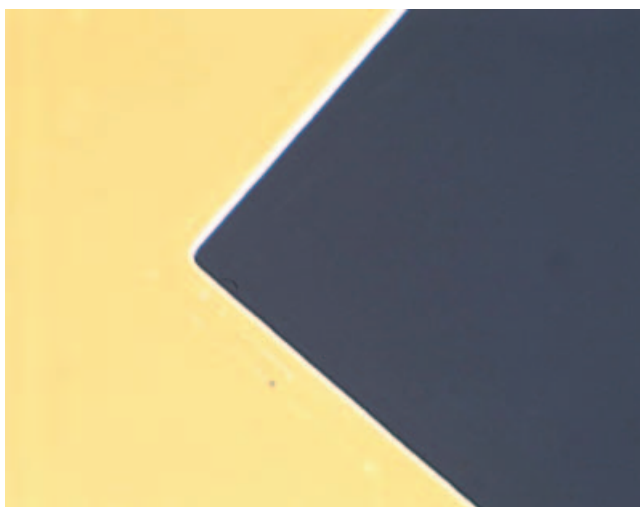
Figure 13. Polarized microscope photograph of LC alignment on photoaligned polymerized azo-dye film [11]. The size of the picture is 1mm 2 . Both homogeneous and twist LC alignment looks perfect between crossed polarizers as black and yellow regions.
