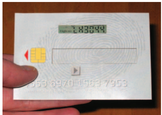
Figure 19. Reflective flexible photoaligned TN-LCD mounted in smart card prototype [38].
