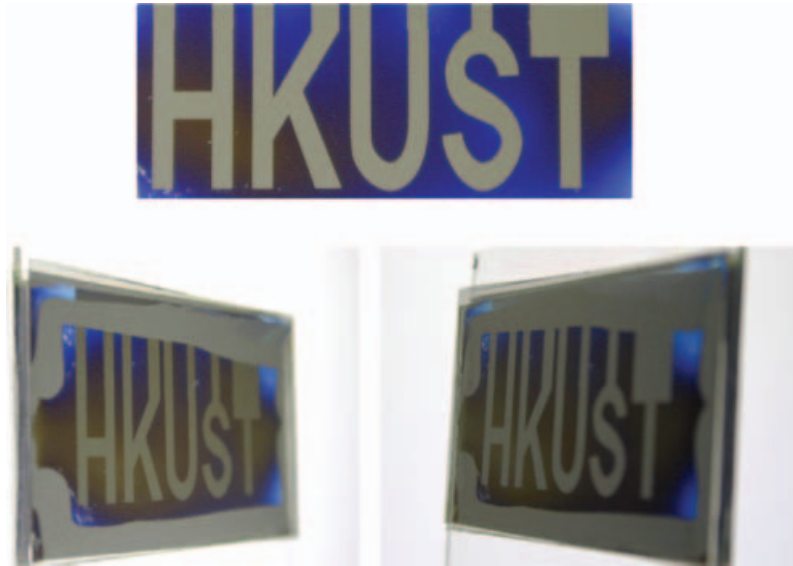
Figure 18. Photo-aligned \pi -BTN liquid crystal display [36].
